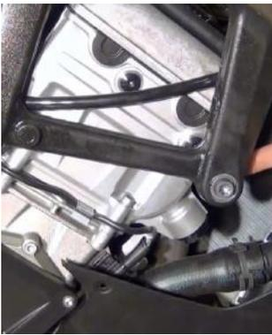
2. Remove the engine stud.
