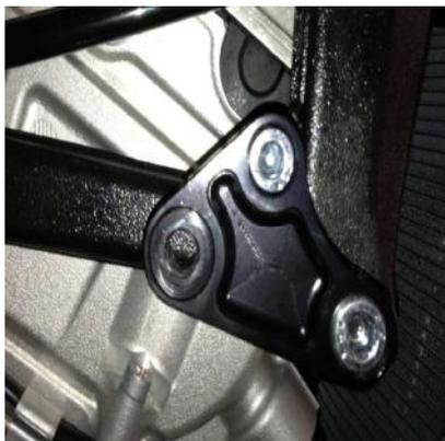
4. The aluminum spacer is bolted to the back of the bracket.
