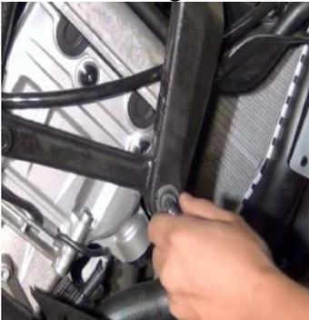
3. Leave conical spacers in the frame. Use M10 x60mm x 1.5 pitch bolt to install the bracket to the motorcycle.
