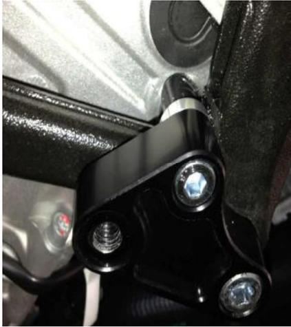
5. Torque down the engine bolt to factory specification.
