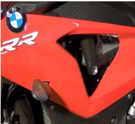
2. Leave conical spacers in the frame. Install long slider on the motorcycle with M10 x90mm x 1.5 pitch bolt.
