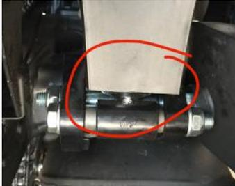
3. Lift the bike from the rearsets using PSR PowerJack or a floor jacks from both side of the bike.
