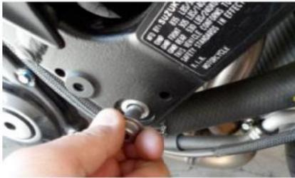
3. Install the bracket using M10 x60 x 1.25 bolt and torque to factory spec.
