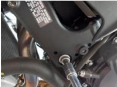
3. Install the Bracket with M10 x60 x 1.25 bolt and torque to factory spec.
