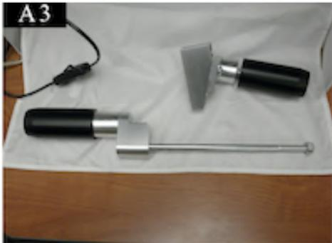
Assemble the left side bracket (shown in Picture A3) using the longer 89.75mm bolt and the 35mm metal spacer. You will place the other spring washer between the head of the bolt and the inside of the slider puck. The long frame bolt should replace the engine frame mount bolt. Slide it through the frame and tighten it down on the other side using the attached nut.
