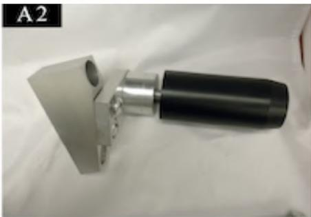
Assemble the right side bracket (shown in Picture A1) using the 24.5mm bolts. Once the bracket is assembled attach the 80mm bolt using the 25mm metal spacer and either frame slider puck, using a spring washer between the bead of the bolt and the inside of the slider puck. This will install on the right side of the frame using the (2) 33.8mm bolts.
