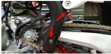
3. Remove M8x35 bolt from the lower chain guide
